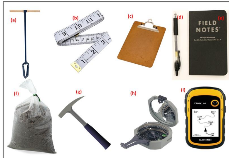
Figure 3. 1 Sampling and geological tools used for the study (a) handheld Auger, (b) Tape measure, (c) Clipboard, ( d-e) Pen and Notebook, (f) 5kg Sample bag, (g) Geological harmer, (h) Campus, (i) Hand-held GPS
