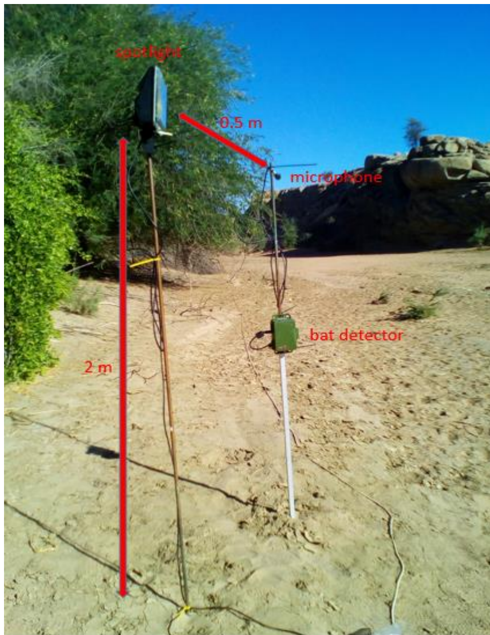
Figure 2.4: Typical site setup along the Kuiseb River, Gobabeb, Namibia. The spotlight and bat detector microphone are at a height of 2 m. The microphone is 0.5 m away from the spotlight.
