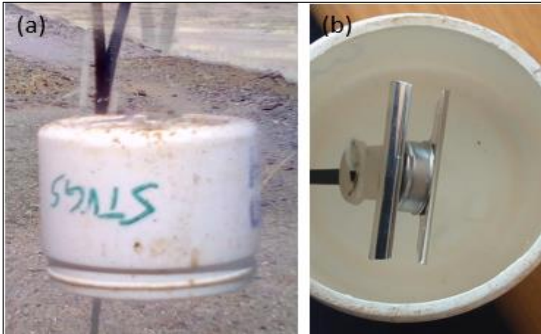
Figure 2.5: A hygrochron iButton temperature/humidity sensor suspended in an open plastic container. Photo (a) shows the suspended container from the side while (b) shows the hygrochron suspended within the container. Care was taken to ensure that the humidity sensor was not obstructed (20 September 2017).
