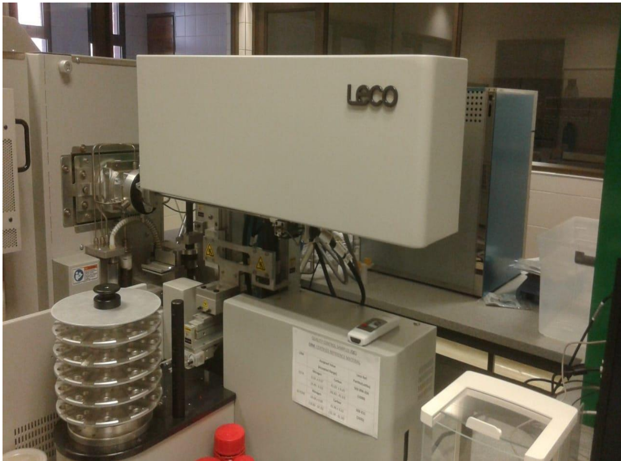
Figure 4.2. LECO Trumac C/N analyser
