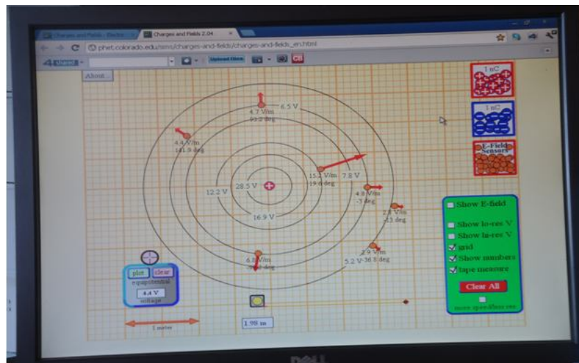
Figure H1: Electric potential and equipotential curves around a positive charge that the students were guided to draw with simulation after their prediction.
