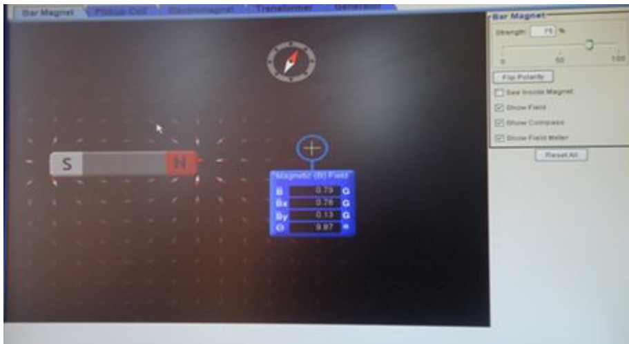
Figure I5: Magnetic field strength of a bar magnet measured with the field meter
