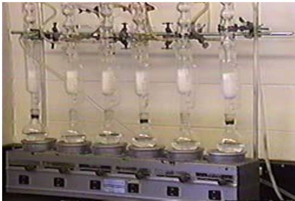
Figure 3.3: Pictorial representation of the Soxhlet extraction process
