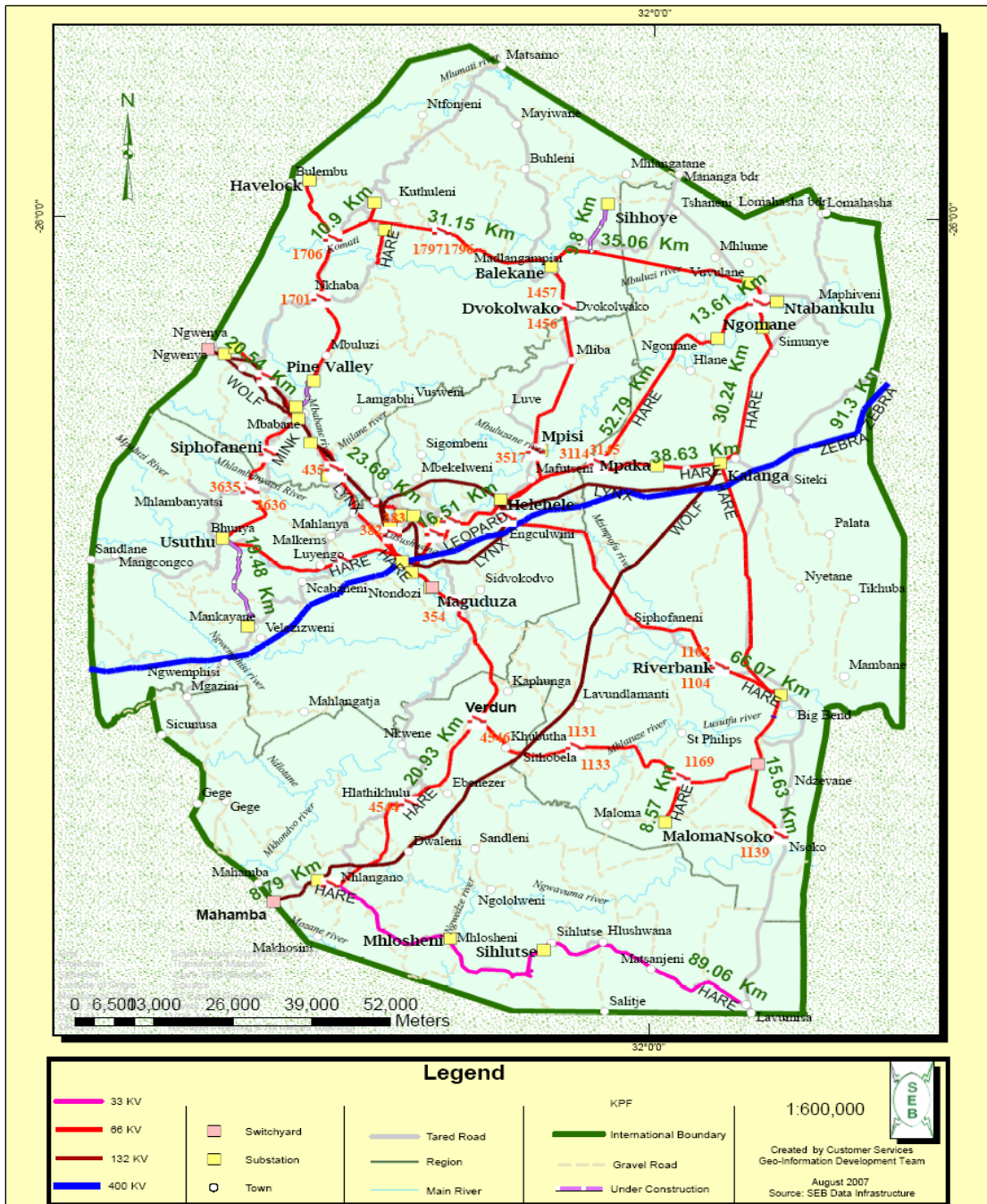
Figure 1.1 Location of power stations and transmission and distribution lines in Swaziland (Source: SEB Drawing Office)
