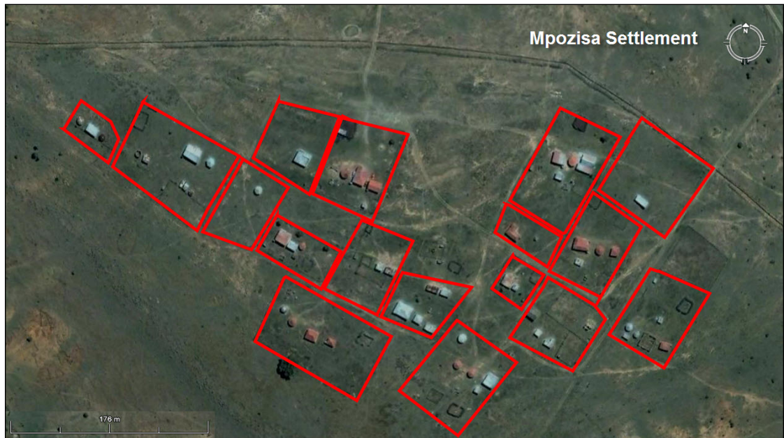
Figure 12 Plots of land that could be identified from the aerial photograph of Mpozisa settlement as being households or homesteads were marked with a red polygon. The red polygons were then summed to establish the number of households or homes in the settlement.
