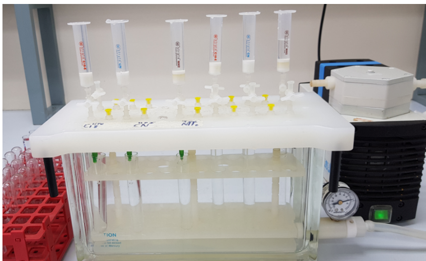
Figure 3-2: Vacuum manifold with SPE cartridges used for m-PRAM
