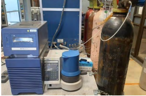
Figure 3.8: IKA oxygen bomb calorimeter apparatus
