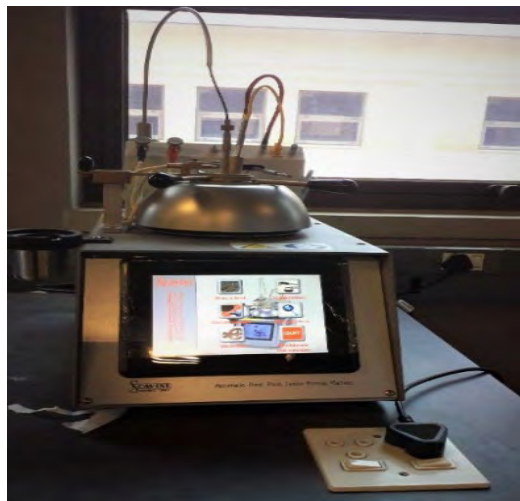
Figure 3.7: Automatic flash point Pensky-Martens apparatus
