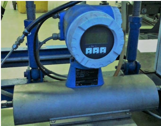
Figure 3.14: Promass 83 fuel meter apparatus and specifications
