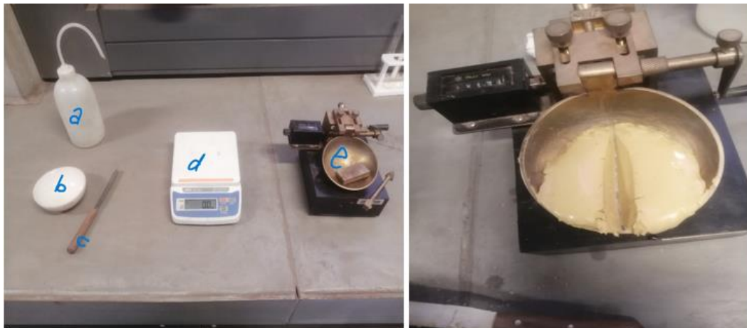
Figure 3.4 (Left) Equipment used for the limit liquid test: (a) water bottle, (b) mixing bowl, (c) spatula, (d) weighing scale (e) Casagrande's cup. (Right) Tailings sample is split at the centre to observe the closing gap when tapping.
