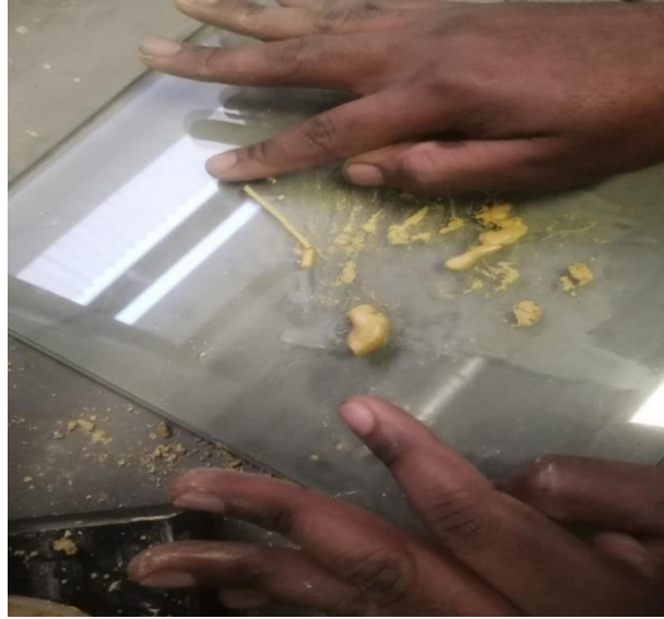
Figure 3.5 Rolling of ellipsoidal paste for determining plastic index.
