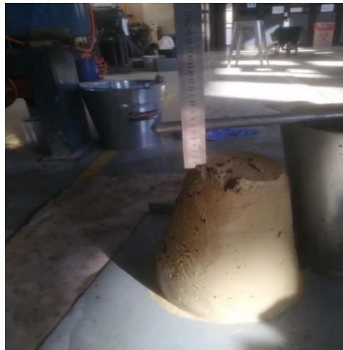
Figure 3.12 The failed slump test due to a stiff mixture
