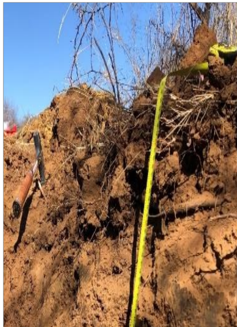
Figure 4.1: Profile pit 2 of a Sterkspuit soil form (SA classification; Solonetz, WRB), with evidence of roots growing horizontally above the prismatic subsoil
