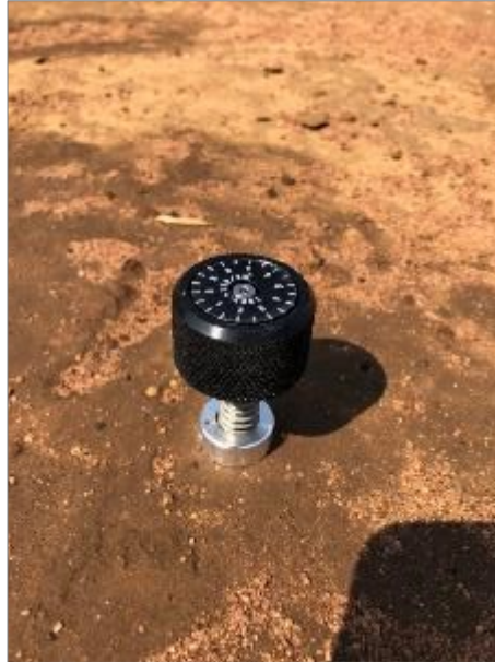
Figure 4.4: The Humboldt H-4212MH pocket shear vane tester (small vanes), pressed into the soil, with blades completely inserted
