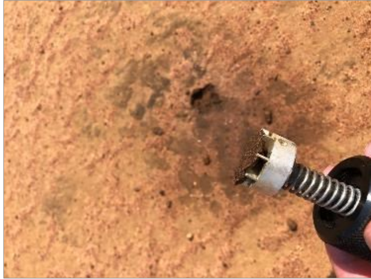
Figure 5.2: Jagged edge hole with scattered pieces of surface crust
