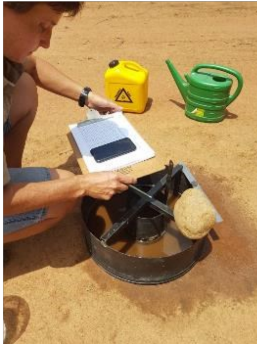
Figure 4.5: The first experiment with the boot rubber on the infiltrrometer (photo credit Dr GP Nortjé)
