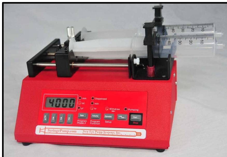
Figure 3.1: NE-8000 High pressure syringe pump (KF Technology) electrospinning set-up.
