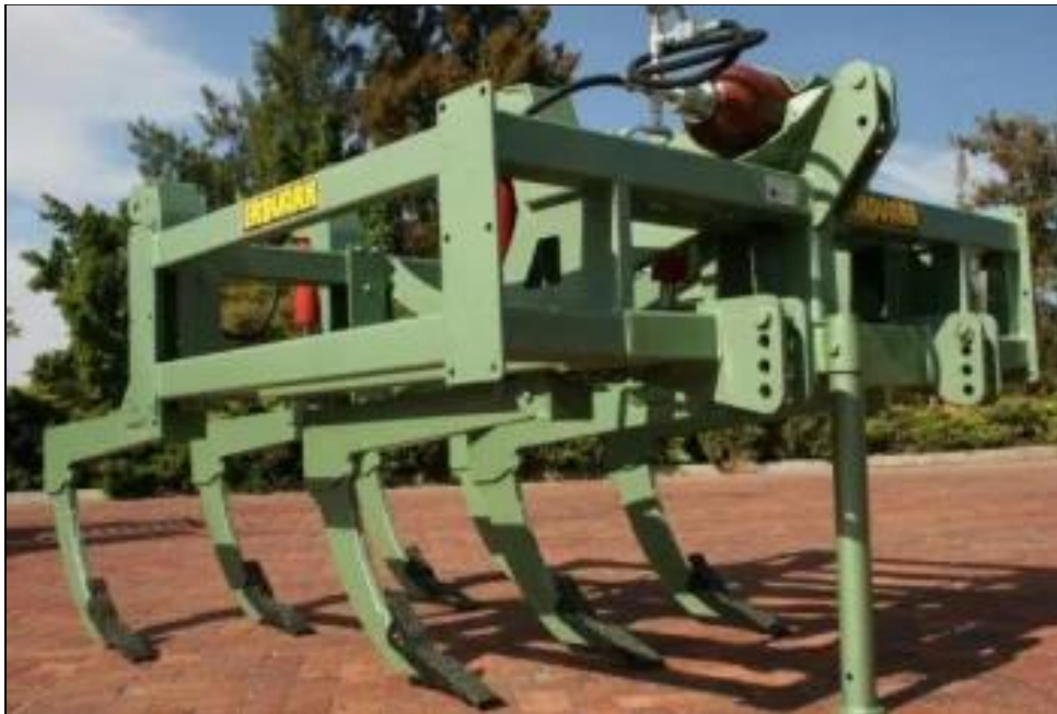
Figure 3.9: Erdvark harvester used in harvesting/ lifting garlic bulbs from the soil.
