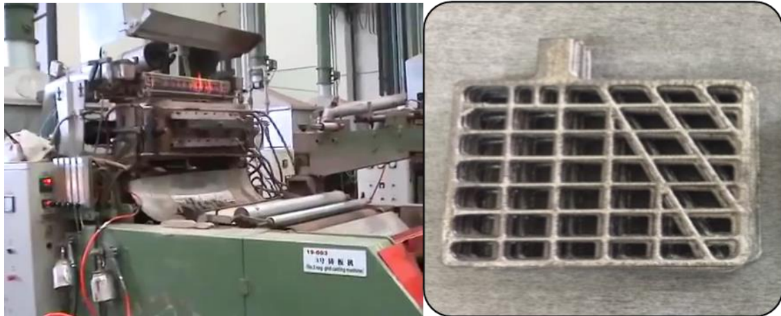
Fig. 6.3 Gravity casted regular lead grids.
