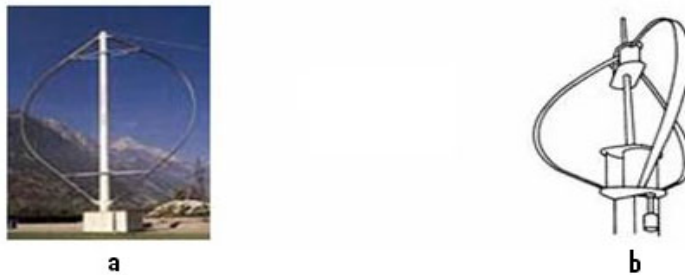
Figure 2. Image of a Darrieus wind turbine (a) and the schema of the Darrieus rotor (b)[12].
