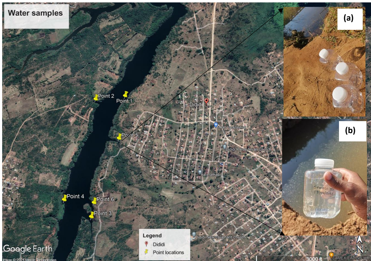
Figure 3.3: Distribution of sample locations and picture inserts (a) and (b) bottles used for water sample collection.
