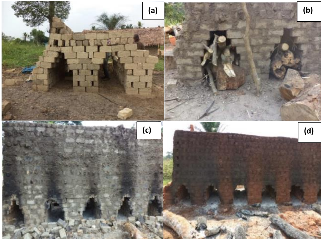
Figure 2.1 Rural clay brick manufacturing process (a) Brick preparation for cooking; (b) Oven; (c) yellow bricks after first cooking and (d) red brick after second cooking.
