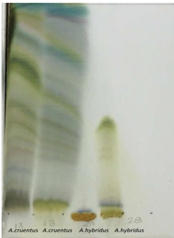
Figure 5.1: TLC chromatogram of crude MeOH leaf extracts of A. cruentus (1 A, B) and A. hybridus (2 A, B). Solvent system- \text{CH}_2\text{Cl}_2 -MeOH (95:5). Detection: Vanillin in sulphuric acid
