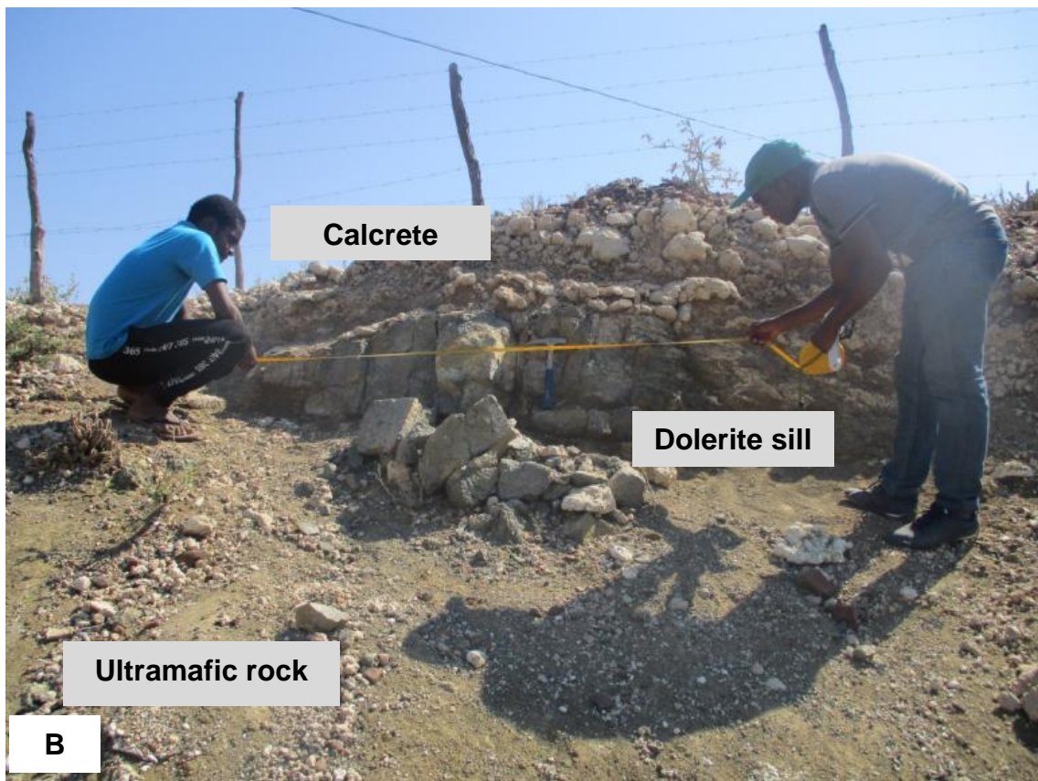
Figure 4.3: Sills (A & B) intruded into the ultramafic rocks in the Venmag Mine. Photographs were taken by the candidate.
