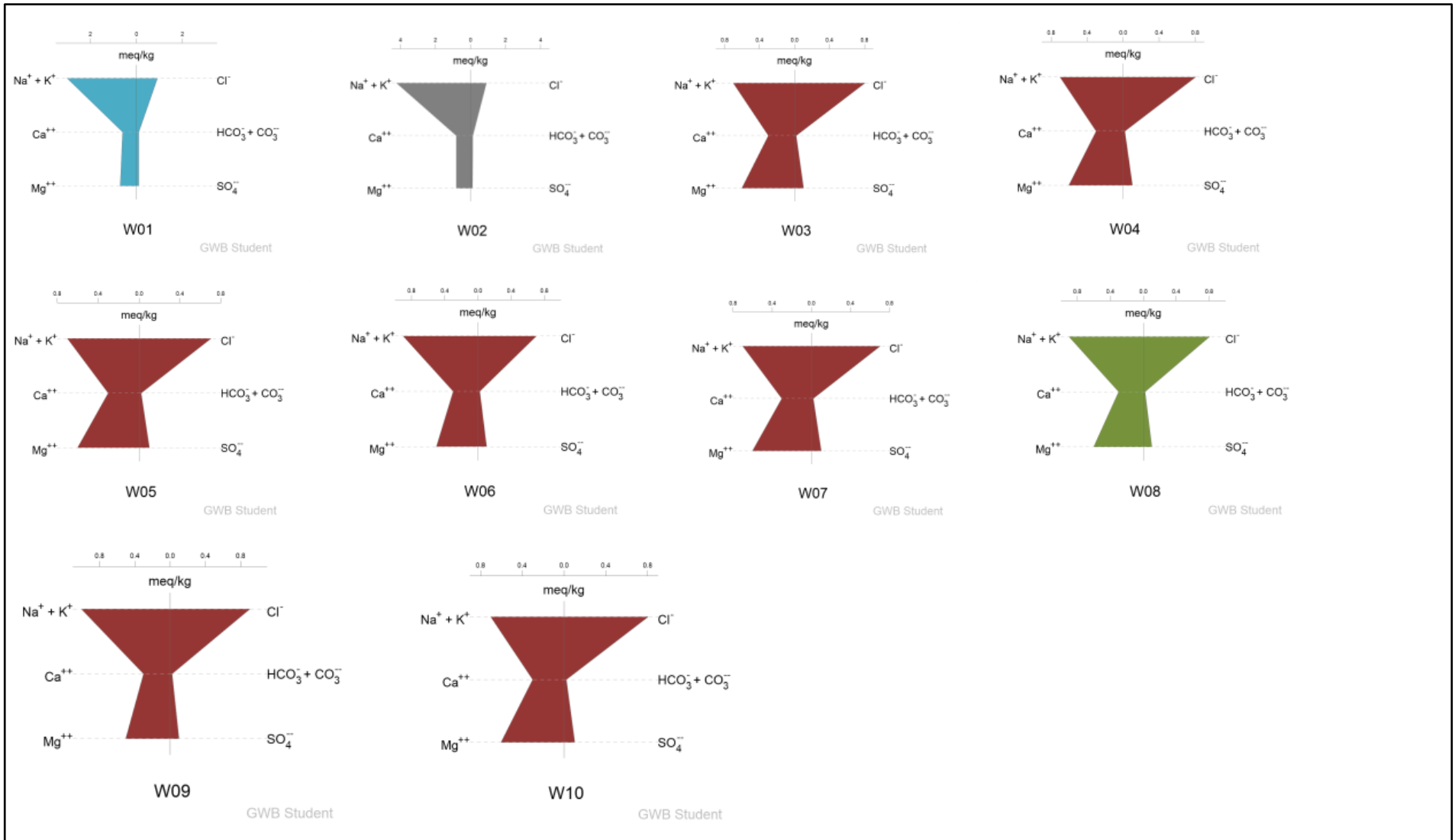
Figure 4.20: Stiff diagrams representing Venmag and Nwanedi River water quality samples (Created by GWB 14 software).
