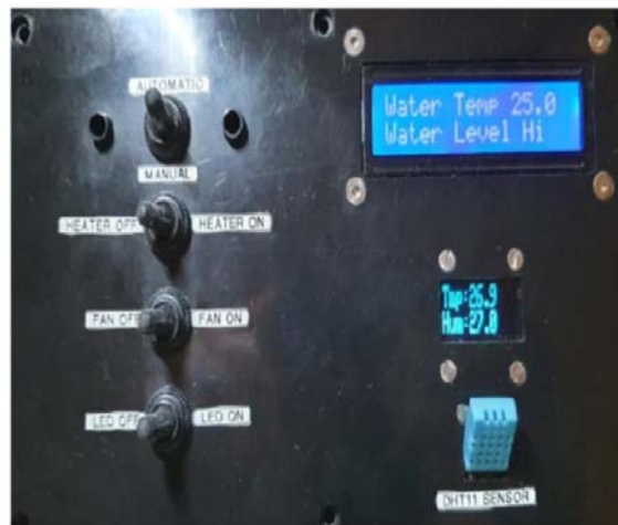
Fig. 6 Final design marine aquarium temperature controller
