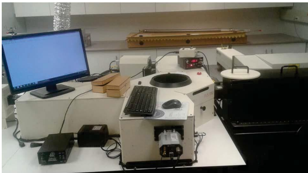
Figure 3.9 A picture of the FLS980 photoluminescence spectrometer; Laser lab 1 University of the Free State (UFS).
