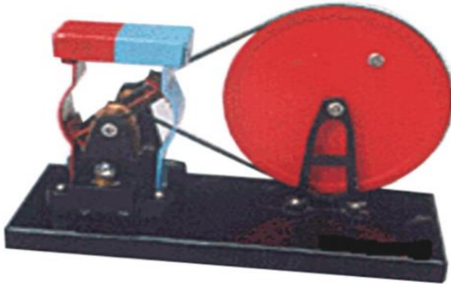
Figure 4.16 A generator model (Source: internet)
