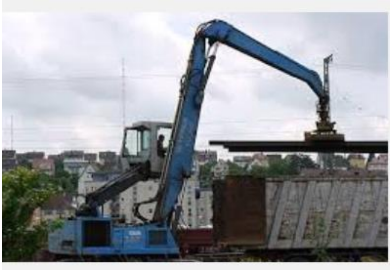
Figure 0.1. An electromagnet used to lift a container from a goods train
