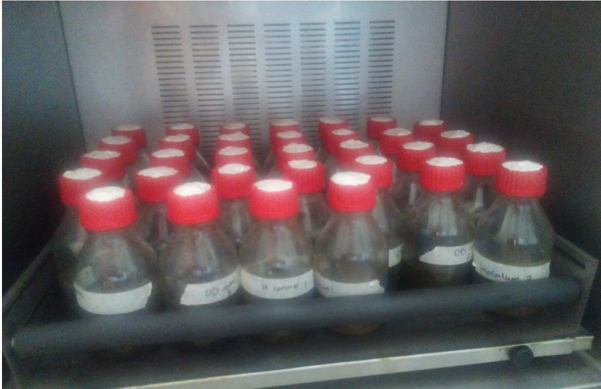
Figure 3.2: Experimental setup of batch AD cultures in a shaker incubator operating at 30°C
