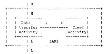
LAPB is substructured into a data\_transfer and timer component, each with their shown interaction points.
