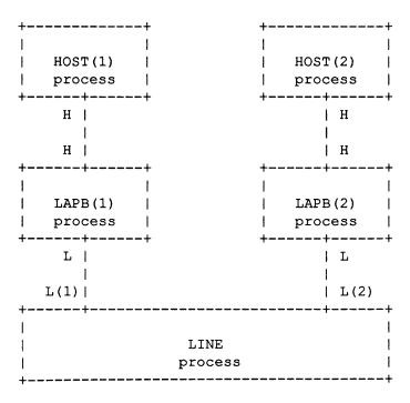
Each LAPB process has a H interaction point to interface to the HOST process (which implies the higher layer protocols) and a L interaction point to interface to the LINE process. Each HOST process has a H interaction point and the LINE process has two interaction points, L(1) and L(2), each to a LAPB process.
