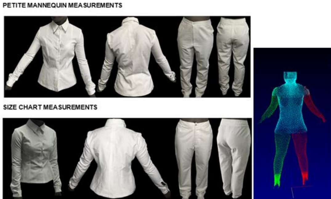
Figure 5.4: The prototype shirt and trouser garments fitted on subject 1 and the subject's 3D full body scan
