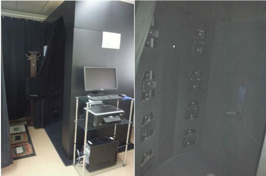
Figure 3.1: Images of the (TC) 2 NX16 3D full body scanner image and the cameras and sensors inside the scanner, captured on the Unisa Science campus scanner laboratory.
