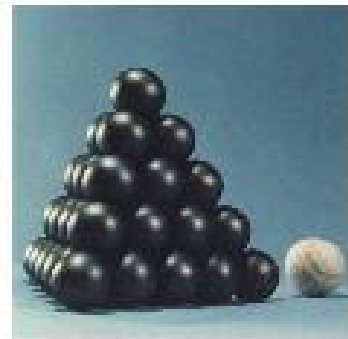
Figure 5–3: Pebble bed reactor ceramic-encapsulated uranium fuel and fuel spheres
