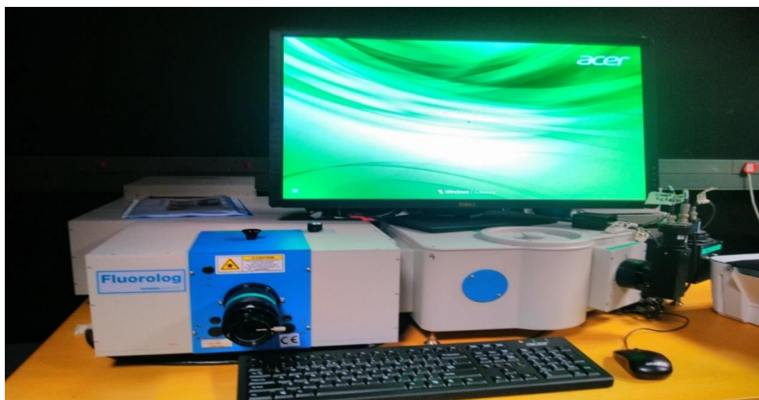
Figure 3.14: Image of Photoluminescence (PL) used in this work
