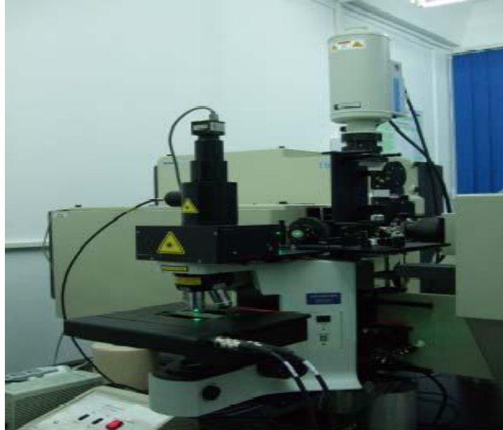
Figure 3.11: A picture of Jobin Yvon T64000 Raman spectrometer
