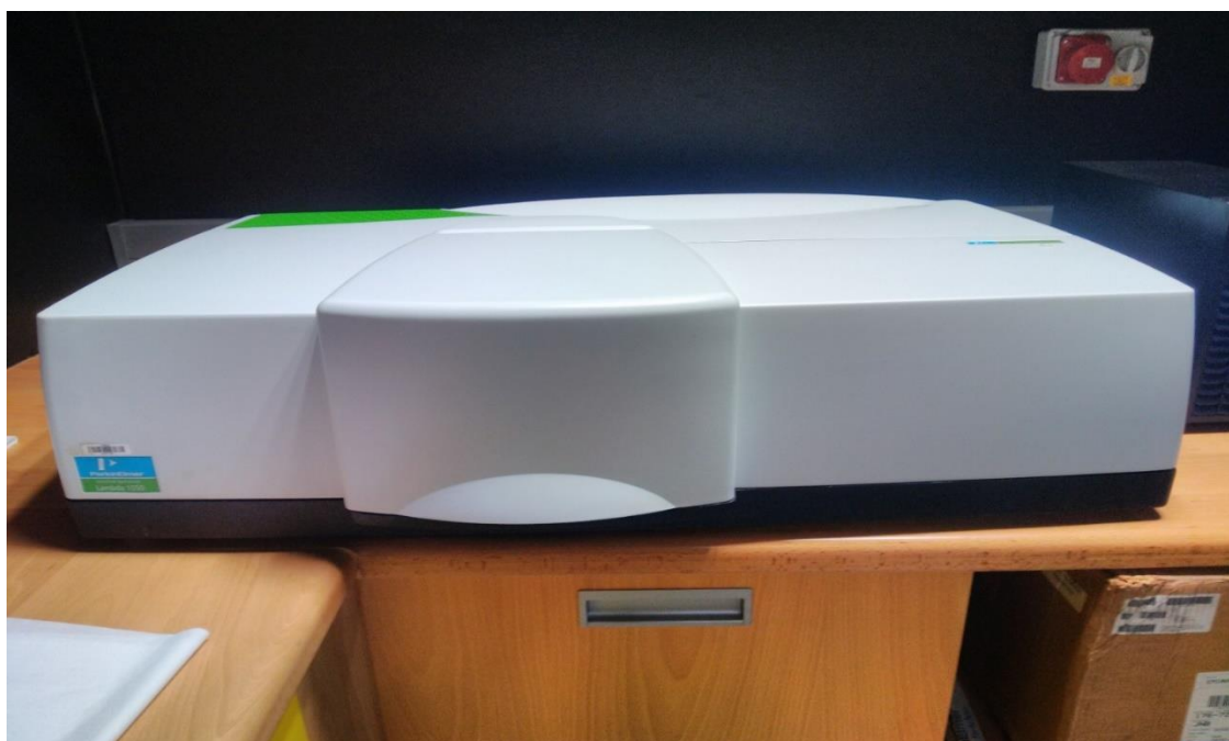
Figure 3.8: A Picture of PerkinElmer Lambda 1050 UV-vis spectroscopy.
