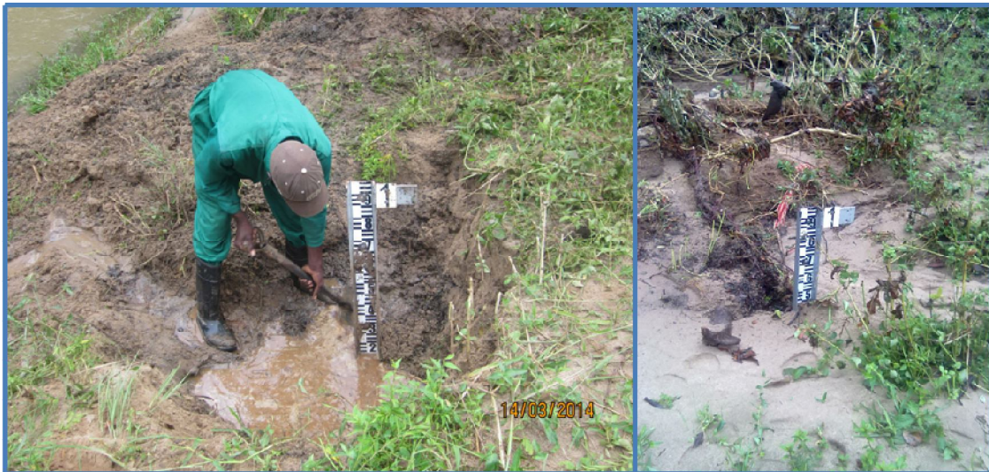
Figure 4.3: Gauging plates silted up at F24 Hydrological Station ( Source: Field surveys )
