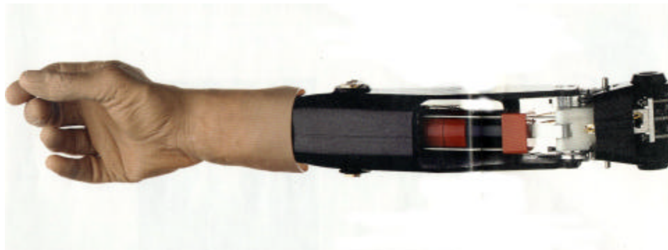
Fig. 4.13 Bionic arm created by the Edinburgh Infirmary's Bioengineering Centre, Benetton's Colors Dec 1996-Jan 1997(18):6-7
