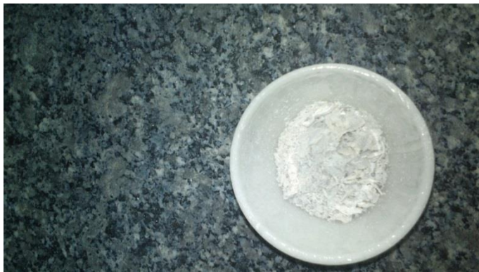
Figure 12: Photograph of Vegetable ash remaining in crucibles following ashing of moringa leaves. Source: Photograph taken by author.
