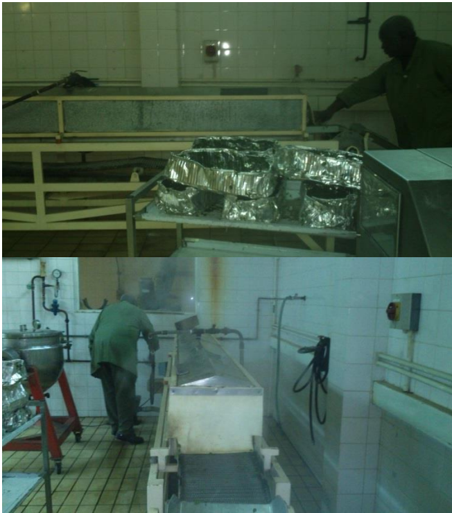
Figure 7: Industrial steam tunnel blanching
