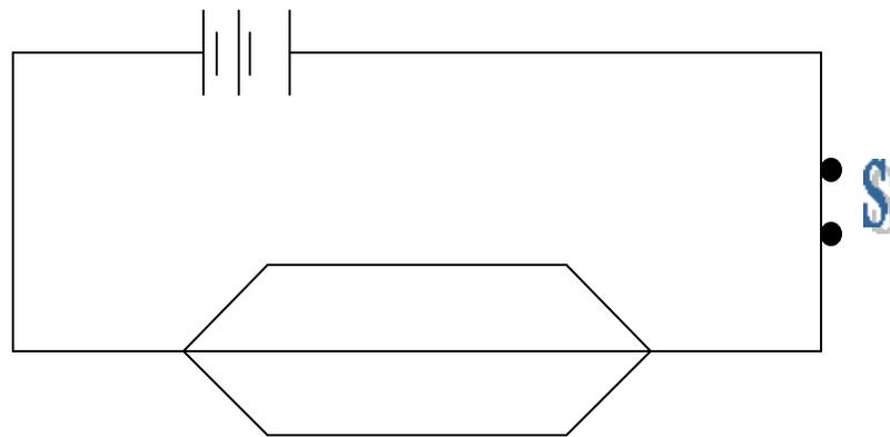
6.3 Parallel circuit, it has the advantage that if one bulb is out of order or not functioning the other bulbs are not affected.
