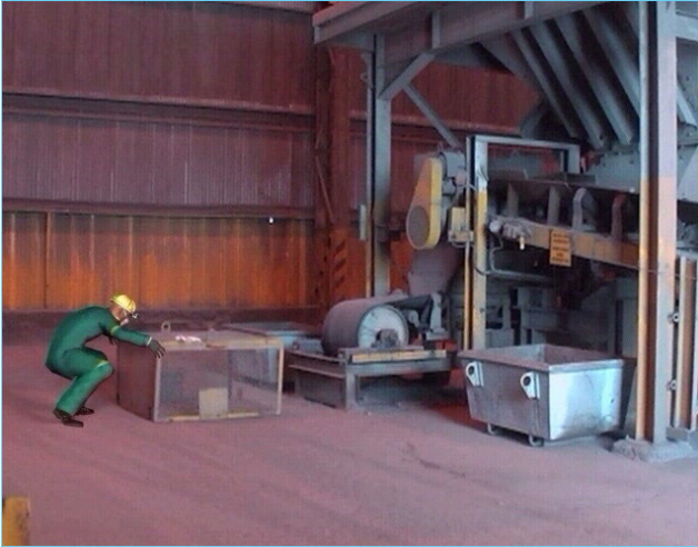
Figure 8. Worker removing the drum guard while conveyor is running.
