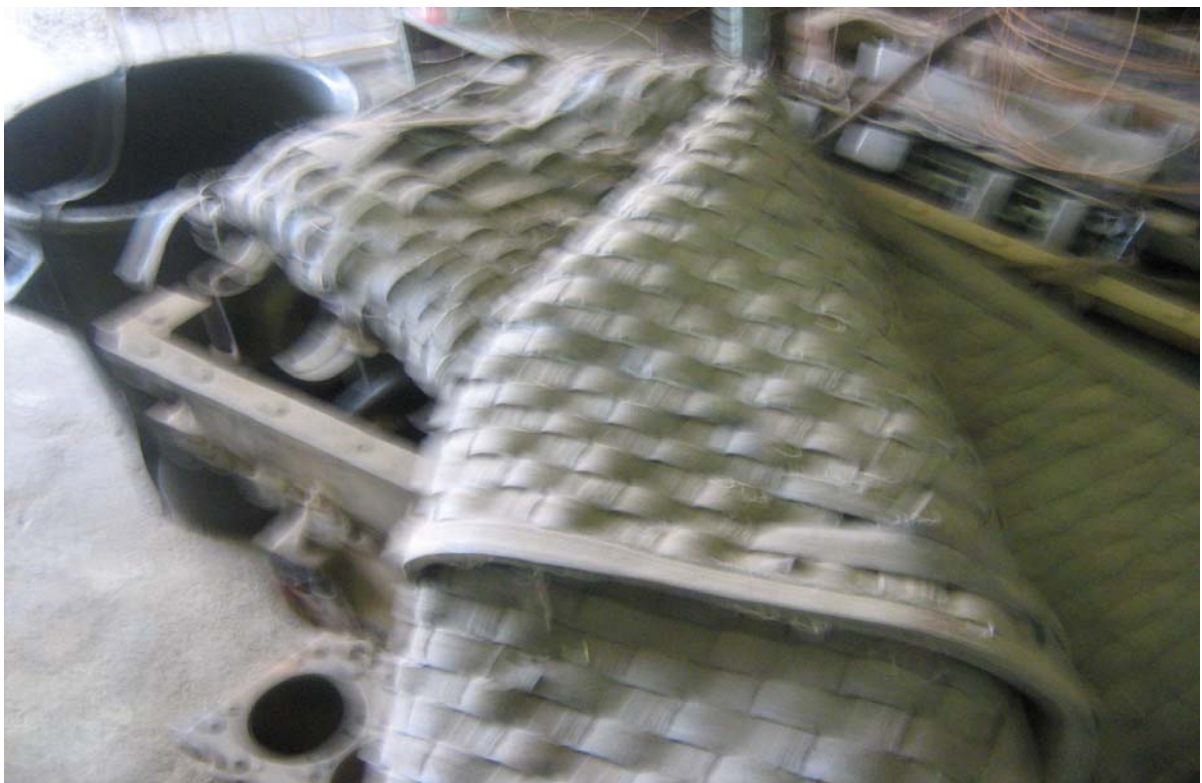
Fig. 6: Rubber mats made from waste tyres; (Source: picture taken from a local company, 2008)
