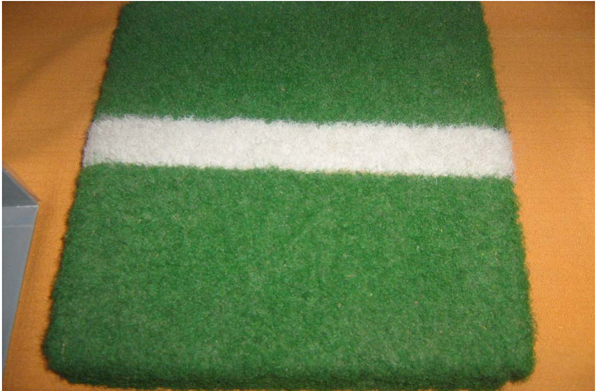
Fig 5: Floor mat and turf made from waste tyres; (Source: picture taken from a local company, 2008)
