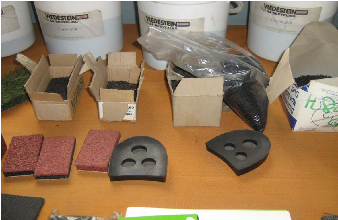
Fig. 9: Various products made from waste tyres; (Source: picture taken from a local company, 2008)
