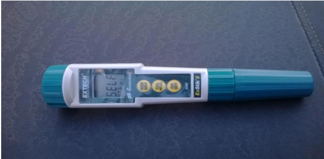
Figure 4.3: The portable ExStik EC500 pH\Conductivity meter.
