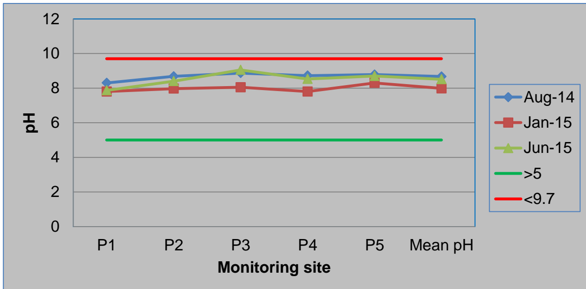
Figure 6.2: In situ pH at monitoring sites measured against drinking water quality standard.
